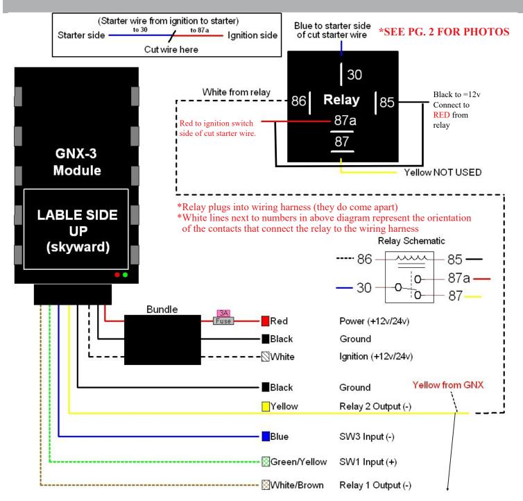
Yellow wire from GNX is the only wire pertinent to the starter interrupt install. For purpose of starter interrupt, ignore all other wires shown on this diagram, as they are used for other functions.
